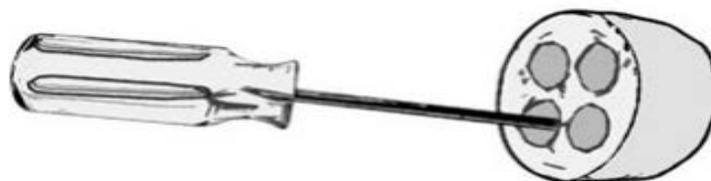
5. Pull 2 inches (5 cm's) of lead wire through the membrane for each one of the cables to be connected to the Multi-Channel Cable Node. Ensure that the number of membranes punctured matches the number of cables to be connected with a maximum of four cables per strain relief with one per membrane for a total of eight cables per Multi-Channel Cable Node.
