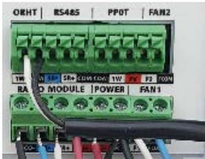
7. Secure the INT2 cable between the Weather Station (ORHT) and the Fan Node enclosure using the P Clips provided. The INT2 cable should be secured roughly every 4 feet (1.25 meters).
