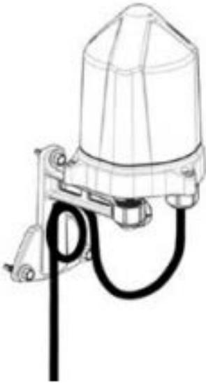
5. Run the Ethernet cable from the Gateway Node to the Power Panel Enclosure. Run the cable into the Power Panel Enclosure box through the strain relief opening on the bottom of the Enclosure. Plug the Ethernet cable into the POE1 connection port on the power supply. Tighten the strain relief clockwise to keep water out of the Enclosure box.
