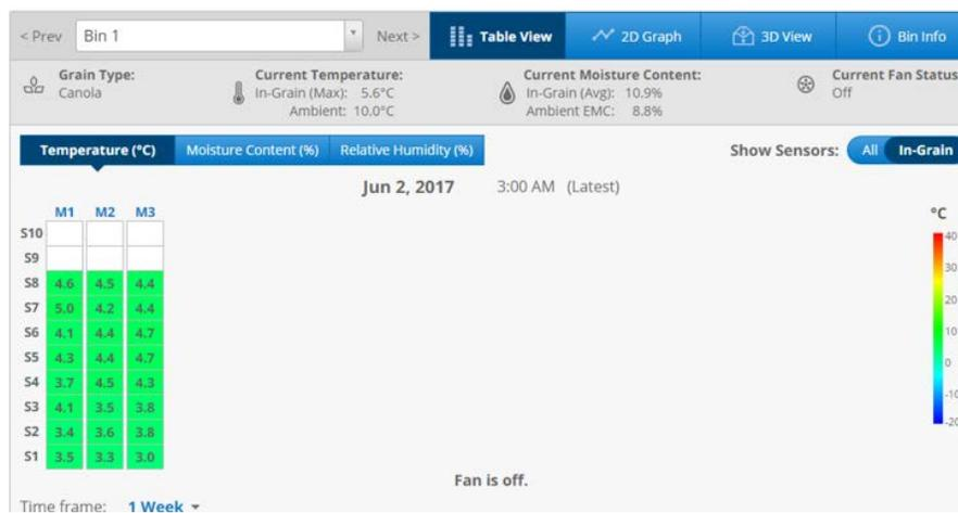
For bins that have moisture cables installed, in addition to being able to view temperature data the humidity data and moisture data are also available to be displayed. For moisture data to appear a Grain Curve must be selected. To add a Grain Curve, go to **System Settings** → **Bins** → (Select Bin) **Grain Info** → **Edit**.
